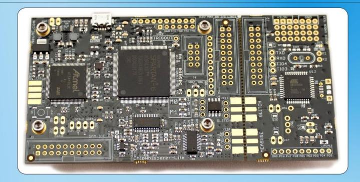
To test the attack, they use a **Chipwhisperer-lite board**, which has a Cortex M4 CPU, which they downclock to 24Mhz. Power usage is sampled at 24Mhz, with high 10-bit precision.
